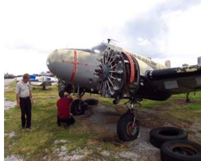
Above: NAA Students working on Landing Gear of C-45H Beechcraft.
